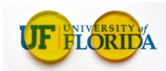
Figure 3. PMMA monoliths containing p -phenylenevinylene platinum(II) acetylide complexes for optical power limiting applications: (left) crossTPV1-DPAF and (right) TPV2-T2.
